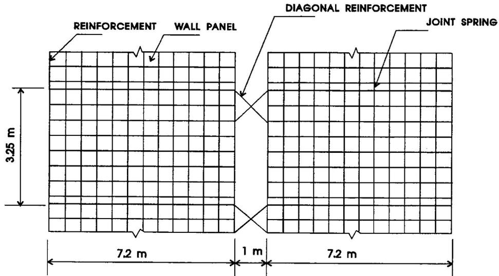
Figure 2. Finite element discretization of the 10-storey structure
