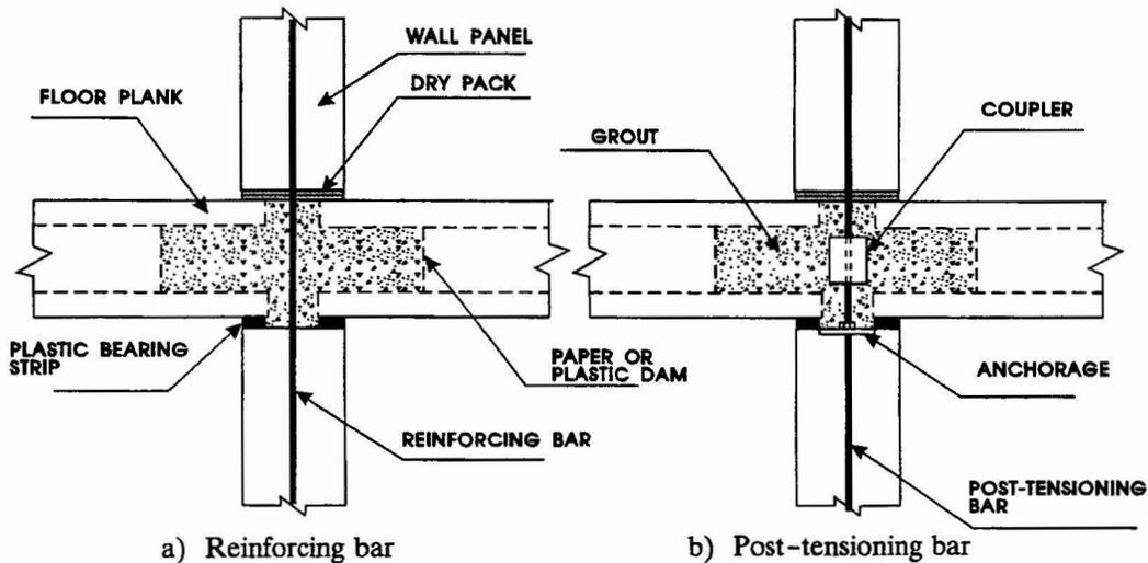
Figure 1. Platform connection details
